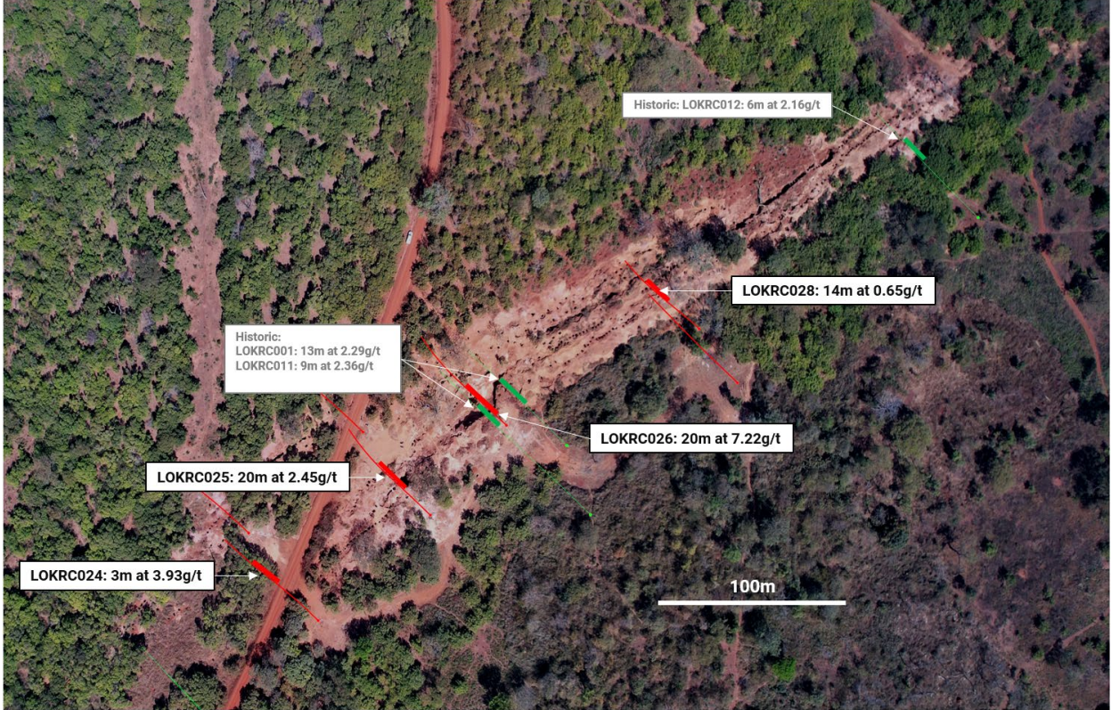
Figure 3: Aerial Photo of Lokolo Main Showing Artisanal Working and Drill Results
